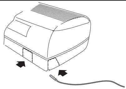
**Installing the SA5 probe on the OMNIA UL / ULI models:**
