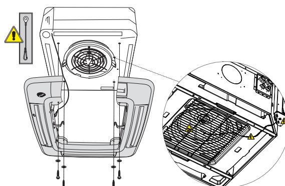
**Installing the SA5 probe on the FCW and FCWI models:**
